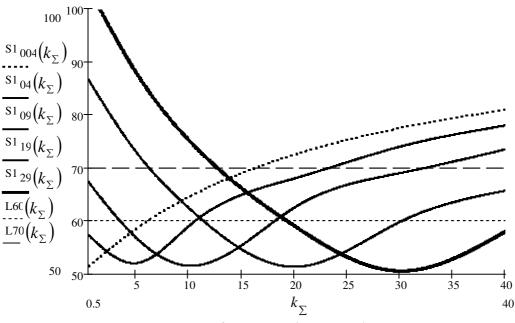
Fig. 3. Dependence of wheel maximum tension on  $k_{\Sigma}$
