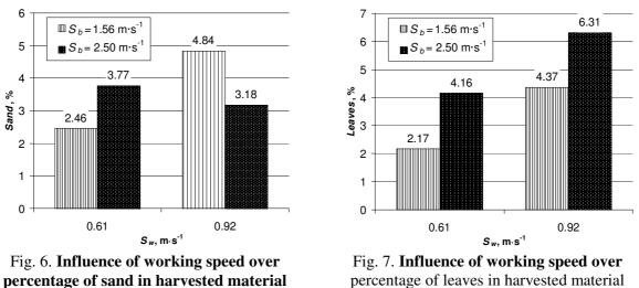
The data processing shows that the percentage of impurities in the harvested material increases in direct proportion to the two parameters (working speed and linear speed of the belts).
