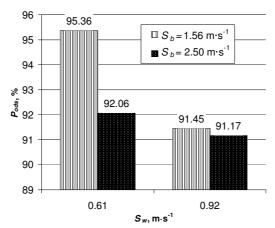
Fig. 5. Influence of working speed over percentage of pods in harvested material
