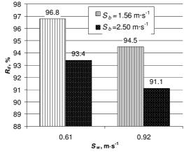
Fig. 2. Influence of machine moving speed over pod removing degree
