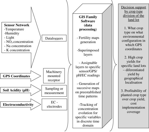
Fig. 2. Logic scheme of the SIGAA decision support system
