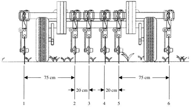
Fig. 1. Veris Technologies 3100 soil electrical conductivity (EC) mapping system: 2, 5 – voltage injector electrodes; 1,6; 3,4 – voltage drop measure electrodes; 1-2, 5-6 – deep soil profile; 2-3, 5-4, – shallow soil profile [3]
