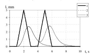
Fig. 5. Impact of inappropriately chosen or damaged input element of measuring system: 1 – real signal; 2 – measured signal; 3 – measured a periodic signal
