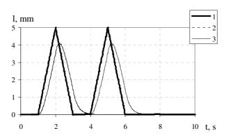
Fig. 6. Impact of appropriately chosen input element of measuring system: 1 – real signal; 2 – measured signal; 3 – measured a periodic signal
