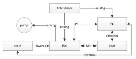
Fig. 4. Communication scheme in system with PC
