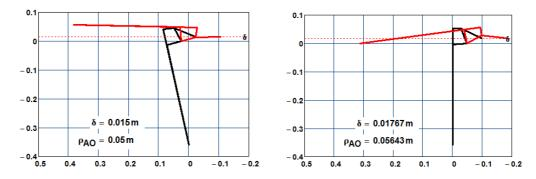
Fig. 4. Positions of virtual manipulator before (left) and after optimization (right)
