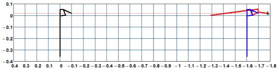
Fig. 6. Positions of virtual manipulator at the initial position and after making a full working cycle (left) and after finishing the returning stroke and turning to the working position (right)
