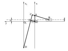
Fig. 10. Manipulator, driven by two dependent drivers
