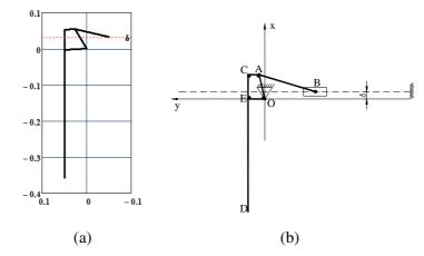
Fig. 3. Virtual model (a) and computational scheme (b) of the manipulator in Fig. 2: O, A, B – pivots; OACED – rigid link
