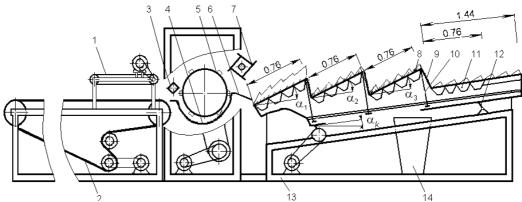
Fig. 1. Test rig scheme of grain separation: 1 – band conveyor for grains, 2 – band conveyor for straw, 3 – feeder, 4 – concave, 5 – threshing cylinder, 6 – grate bars, 7 – beater, 8 – sections of straw walker, 9 – steps of straw walker, 10 – inclination control screws of the straw walker sections, 11 – sample bags, 12 – crankshafts, 13 – straw walker frame, 14 – grain collection bag, α<sub>1</sub>, α<sub>2</sub>, α<sub>3</sub> –
