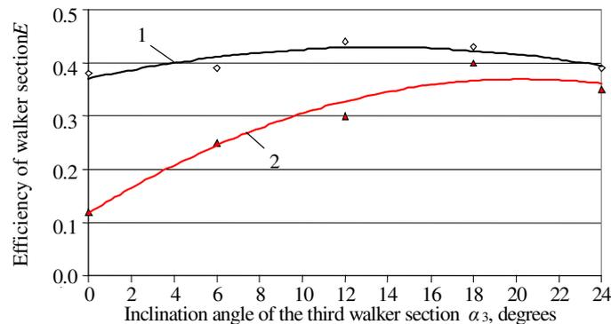
Fig. 7. The impact of the inclination angle of the third sections ( $\alpha_3$ ) of the straw walker on the efficiency coefficient ( $E$ ) of the third (1) and the fourth (2) sections, when:  $\alpha_1=22^\circ$ ,  $\alpha_2=10^\circ$ ,  $\alpha_4=0^\circ$ ;
