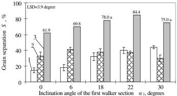
Fig. 3. The impact of the inclination angle of the first sections ( $\alpha_1$ ) of the straw walker on the sum grain separation (S) through the first (1) and the second (2) sections, and the three sections (3) of the straw walkers ( $L_{3d}$ =2.28 m), when: n=215 min<sup>-1</sup>,  $\alpha_2$ = $\alpha_3$ =0°
