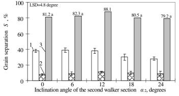
Fig. 4. The impact of the inclination angle of the second sections ( $\alpha_2$ ) of the straw walker on the sum grain separation (S) through the second (1) and the third (2) sections, and the three sections (3) of the straw walkers ( $L_{3d}$ =2.28 m), when:  $n_k$ =215 min<sup>-1</sup>,  $\alpha_1$ =22°,  $\alpha_3$ =0°
