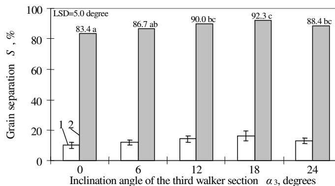
Fig. 6. The impact of the inclination angle of the third sections ( $\alpha_3$ ) of the straw walker on the sum grain separation ( $S$ ) through the third and the fourth (1), and the three sections (2) of the straw walkers ( $L_{3d}=2.28 \text{ m}$ ), when:  $n=215 \text{ min}^{-1}$ ,  $\alpha_1=22^\circ$ ,  $\alpha_2=10^\circ$ ,  $\alpha_4=0^\circ$
