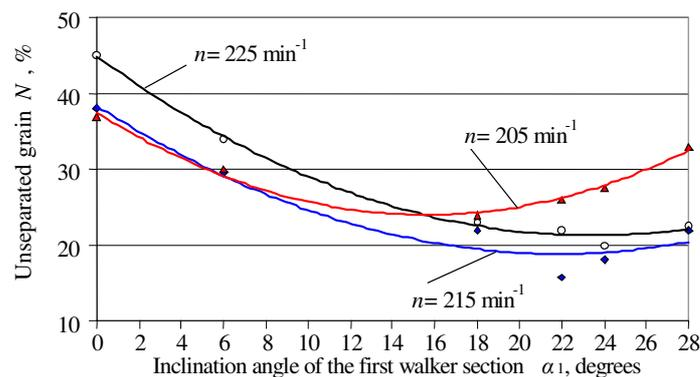
Fig. 2. The impact of the inclination angle of the first sections ( $\alpha_1$ ) of the straw walker and the crankshaft rotational speed ( $n$ ) on the grain amount ( $N$ ) remaining in the straw behind the three sections of the straw walkers ( $L_{3d}=2.28$  m), when:  $\alpha_2=\alpha_3=0^\circ$
