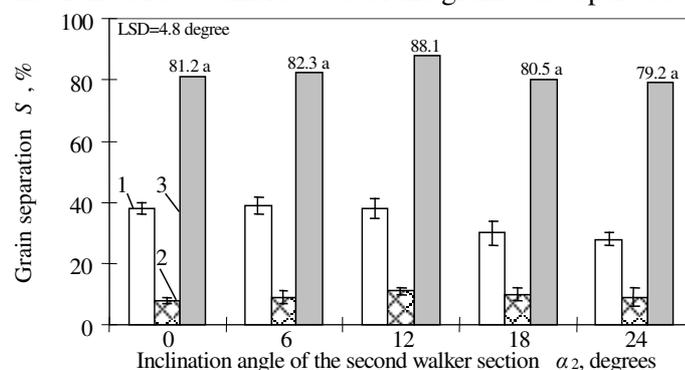
Fig. 4. The impact of the inclination angle of the second sections ( $\alpha_2$ ) of the straw walker on the sum grain separation ( $S$ ) through the second (1) and the third (2) sections, and the three sections (3) of the straw walkers ( $L_{3d}=2.28 \text{ m}$ , when:  $n_k=215 \text{ min}^{-1}$ ,  $\alpha_1=22^\circ$ ,  $\alpha_3=0^\circ$ )
