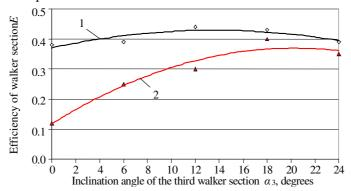
Fig. 7. The impact of the inclination angle of the third sections ( $\alpha_3$ ) of the straw walker on the efficiency coefficient (*E*) of the third (1) and the fourth (2) sections, when:  $\alpha_1=22^\circ$ ,  $\alpha_2=10^\circ$ ,  $\alpha_4=0^\circ$ ;
