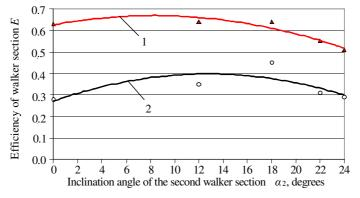
Fig. 5. The impact of the inclination angle of the second sections ( $\alpha_2$ ) of the straw walker on the efficiency coefficient (*E*) of the second (1) and the third (2) sections, when:  $n_k=215 \text{ min}^{-1}$ ,  $\alpha_1=22^\circ$ ,  $\alpha_3=0^\circ$ ; 1 – the efficiency coefficient of the second sections,  $E = -0.0006\alpha_2^2 + 0.010\alpha_2 + 0.63$ ;  $R^2=0.92$ ; 2 – the efficiency coefficient of the third sections,  $E = -0.0008\alpha_2^2 + 0.020\alpha_2 + 0.27$ ;  $R^2=0.84$
