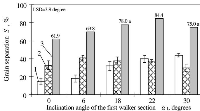
Fig. 3. The impact of the inclination angle of the first sections ( $\alpha_1$ ) of the straw walker on the sum grain separation ( $S$ ) through the first (1) and the second (2) sections, and the three sections (3) of the straw walkers ( $L_{3d}=2.28 \text{ m}$ , when:  $n=215 \text{ min}^{-1}$ ,  $\alpha_2=\alpha_3=0^\circ$ )
