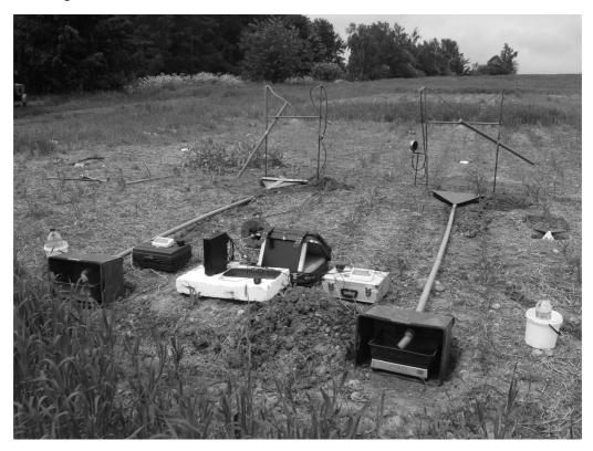
Fig. 1. Measurements by rainfall simulator
