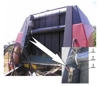
Fig. 1. Location potentiometer on the belt tensioning mechanism: 1 – belt tension roller mechanism; 2 - connecting rod; 3 - potentiometer
