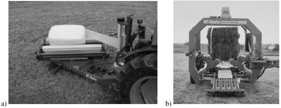
Fig. 1. Wrapping of a square bale with a film ribbon
