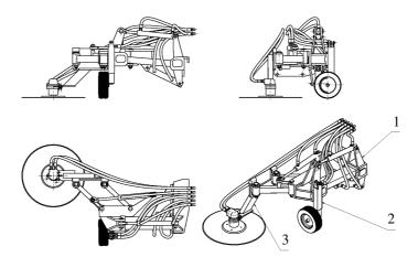
Fig. 5. Complete assembly of cutting mechanism: 1 – Reith interaxle carrier, 2 – copy wheel, 3 – cutting mechanism
