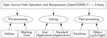
Fig. 2. **OpenFoam toolbox structure:** All data processing and manipulations can be done using a part of this toolbox either with benefits of external programs (e.g., mesh generators, visualisation products, user defined inputs of data ...)
