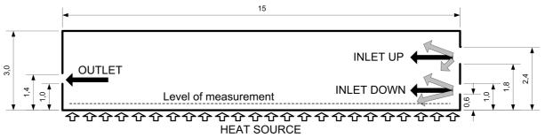
Fig. 1. **Typical geometry used as a student project case:** All distances are given in meters. The level of measurement is the height above the floor, where the measurement at real objects was made. The heat source represents the heat generated by poultry
