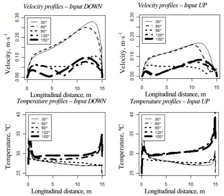
Fig. 5. **Typical results of CFD analysis of variants.** The comparison of the velocity and temperature profiles at the level of measurement. The angle of the input stream is the parameter of these graphs. 90 degrees mean that the input flow is horizontal. Lower angles mean that the intake air goes down; higher values mean that it goes up
