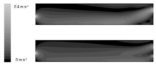
Fig. 4. **Comparison of two velocity profiles for the same flowrate.** The upper corresponds to only the upper window open and the direction of the input stream 60°. The lower case shows the change when both inlets are open and the input stream of the down inlet has the direction 30°.
