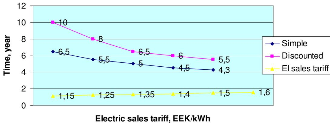
Fig. 2. Payback time dependence on electric sales tariff (on silo price 300 EEK t<sup>-1</sup>)
