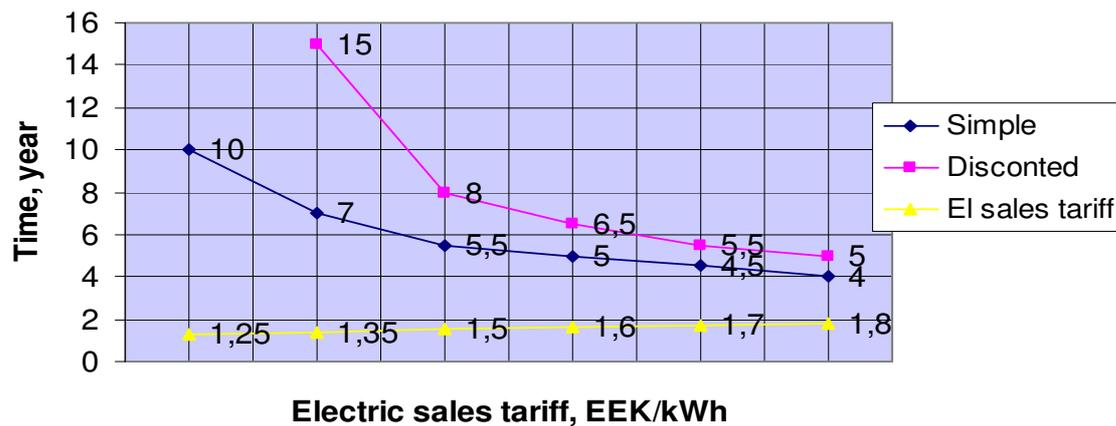
Fig. 4. Payback time dependence on electric sales tariff (on silo price 400 EEK t<sup>-1</sup>)
