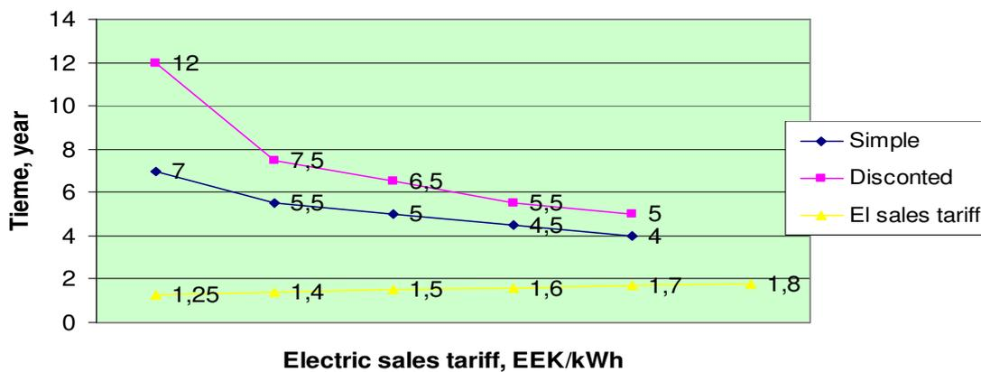
Fig. 3. Payback time dependence on electric sales tariff (on silo price 350 EEK t<sup>-1</sup>)
