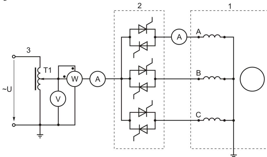
Fig. 1. Asynchronous drive diagram:
