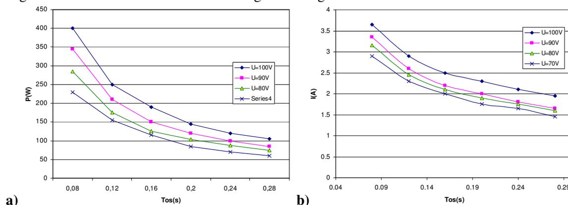
Fig. 5. Consumed power  $P$  and current  $I$  dependent on oscillation period  $T_{OS}$ :
