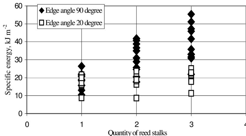
Fig. 3. Reed stalk specific cutting energy consumption
