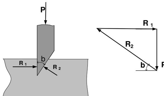
Fig. 5. Reactions for sliding of knife wedge
