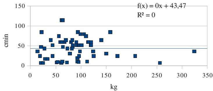
Fig. 4. Time consumption over stump dry-weight for birch stumps, all plots
