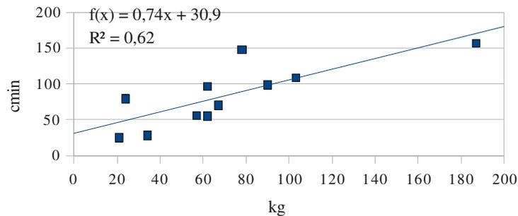
Fig. 5. Time consumption over stump dry-weight for pine stumps, plot No 1
