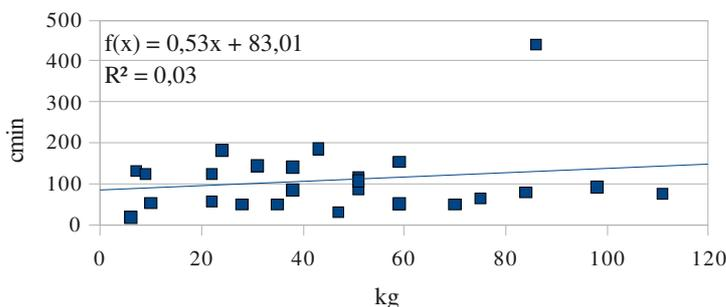
Fig. 2. Time consumption over stump dry-weight for pine stumps, all plots
