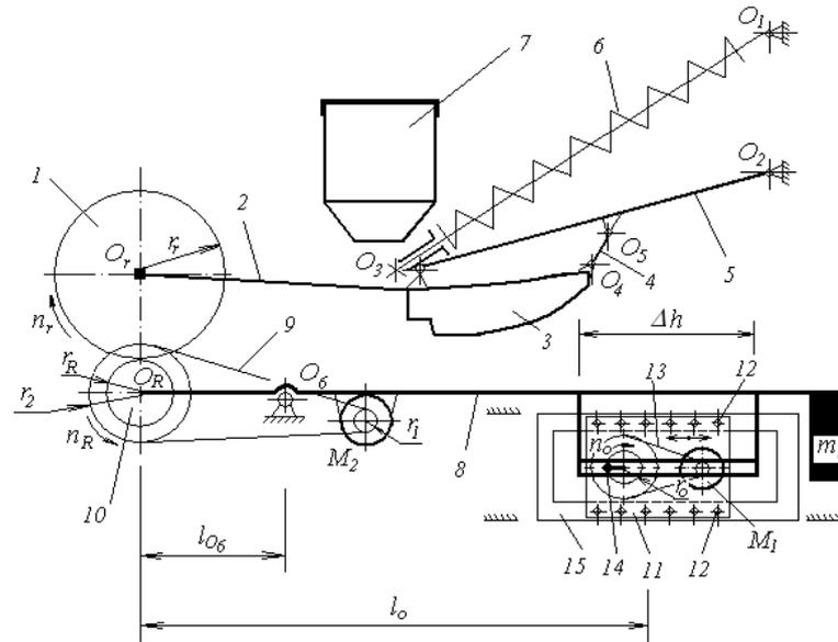
Fig.3. Diagram of the stand for experimental testing of the seeder unit:
