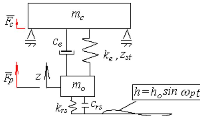
Fig. 2. Equivalent oscillatory dynamic model of the seeder unit for study of forced oscillations produced by the soil profile upon the compaction wheel
