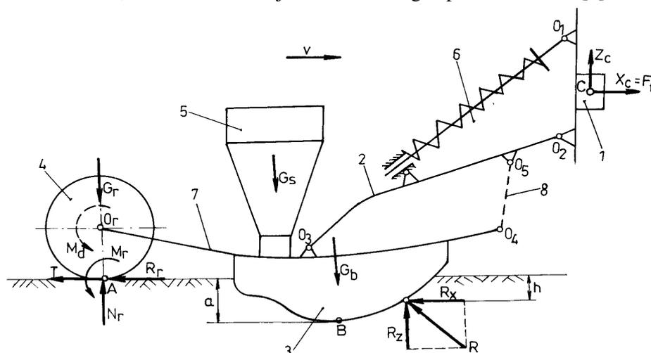
**Fig.1. External forces acting upon the working unit of a precision seeder running at constant speed on horizontal soil**
