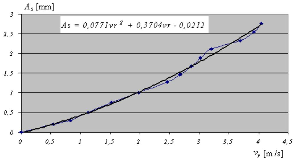
Fig. 4. The dependence of the amplitude of the settling wheel leaps on the running speed at the unit with springs which is subject to oscillations
