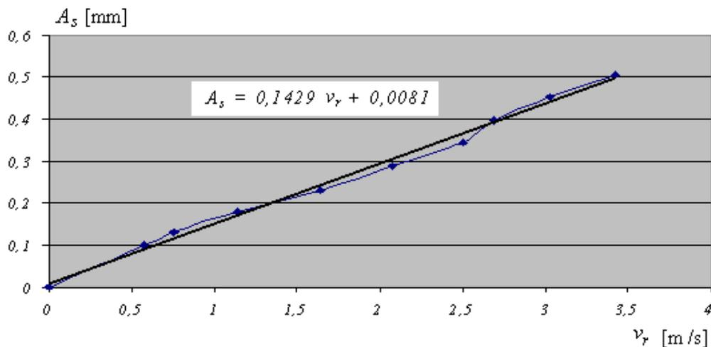
Fig. 5. The dependence of the leap amplitude on the settling wheel speed
