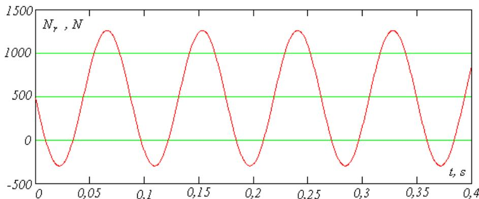
**Fig. 2. Variation of the normal reaction of the soil upon the compaction wheel at the moving speed of the unit with  $v_a = 2.78 \text{ m s}^{-1}$  ( $\approx 10 \text{ km h}^{-1}$ )**
