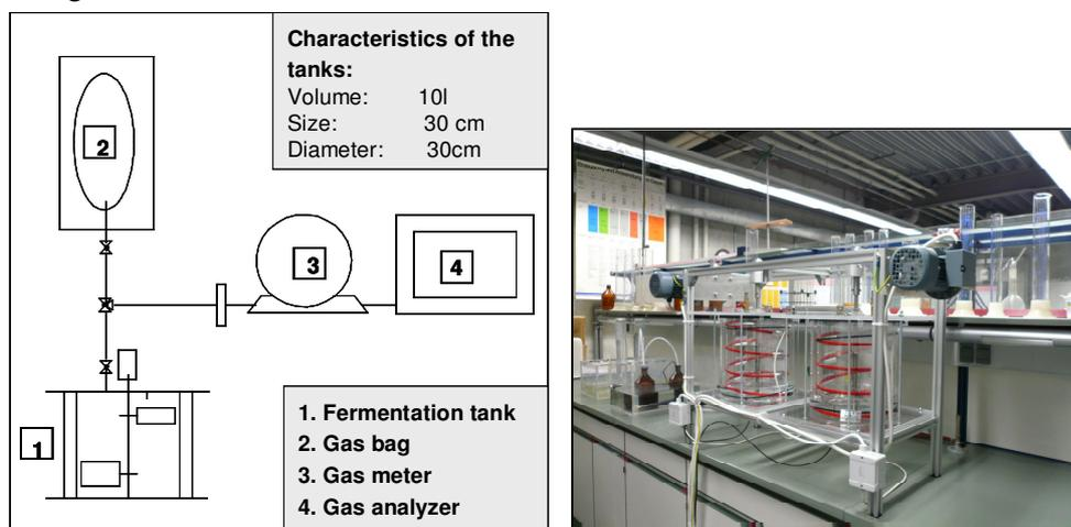
Fig. 2. Test plant for wet fermentation experiments
