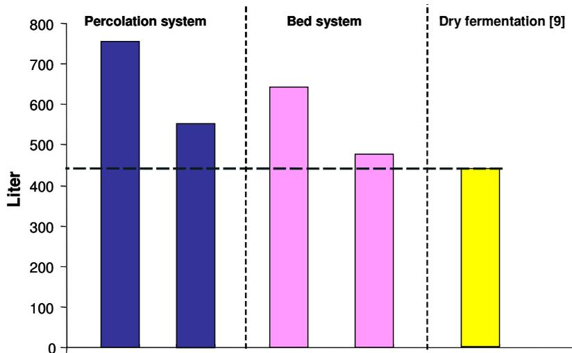
Fig. 4. Biogas yield of the laboratory experiments in comparison with the values found in literature for a retention time of 30 days
