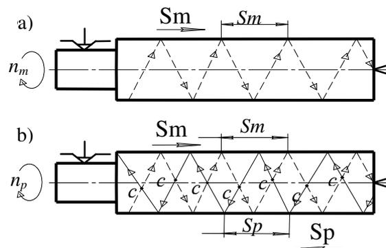
Fig. 1. Diagram of creation of local metastability in the workable material (a) and the blank turning process after preliminary plastic effect on the material (b)
