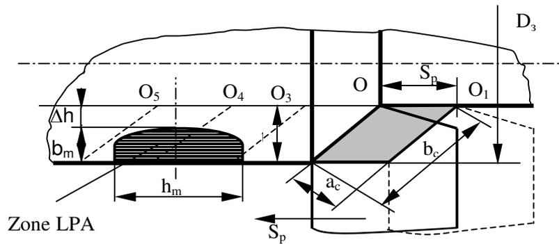
Fig. 2. Diagram of the bilateral layout of the local plastic action zone and area of the transverse cut off layer of the shaving
