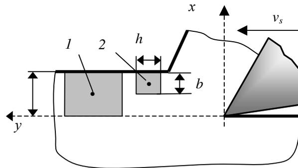
Fig. 3. Diagram of the layout of the local action zones in the cut off layer with different relations of the depth of action  $b$  and of the depth of the cut off layer  $a$ : 1- $b \geq a$ ; 2- $b < a$
