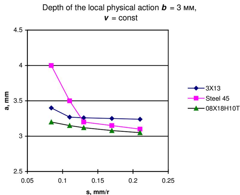
Fig. 4. Area of continuous chip breaking by changes of feed  $s$  for different materials
