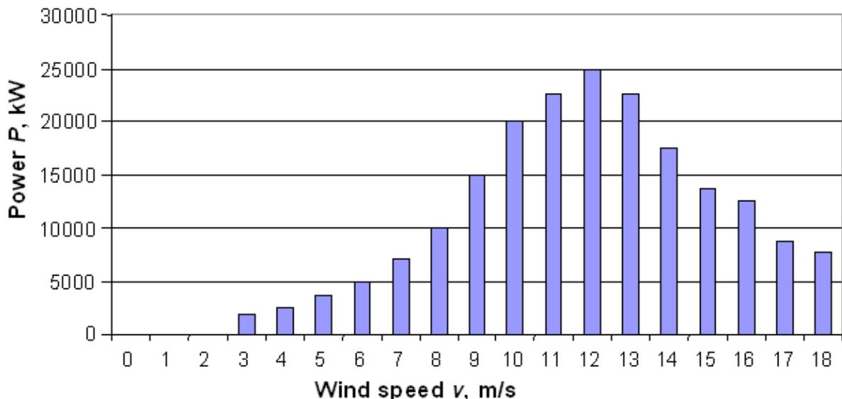
Fig. 4. Wind turbine WP20kW power output depending on the wind speed
