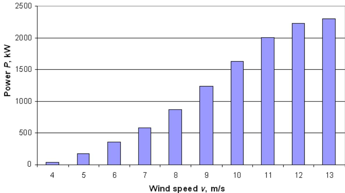
Fig. 3. Nordex 90 wind turbine power depending on wind speed
