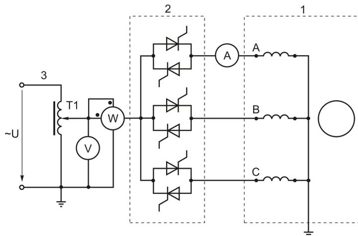
Fig. 2. **Asynchronous motor connection scheme:** 1 – asynchronous motor, 2 – semiconductor switch blok, 3 – autotransformer
