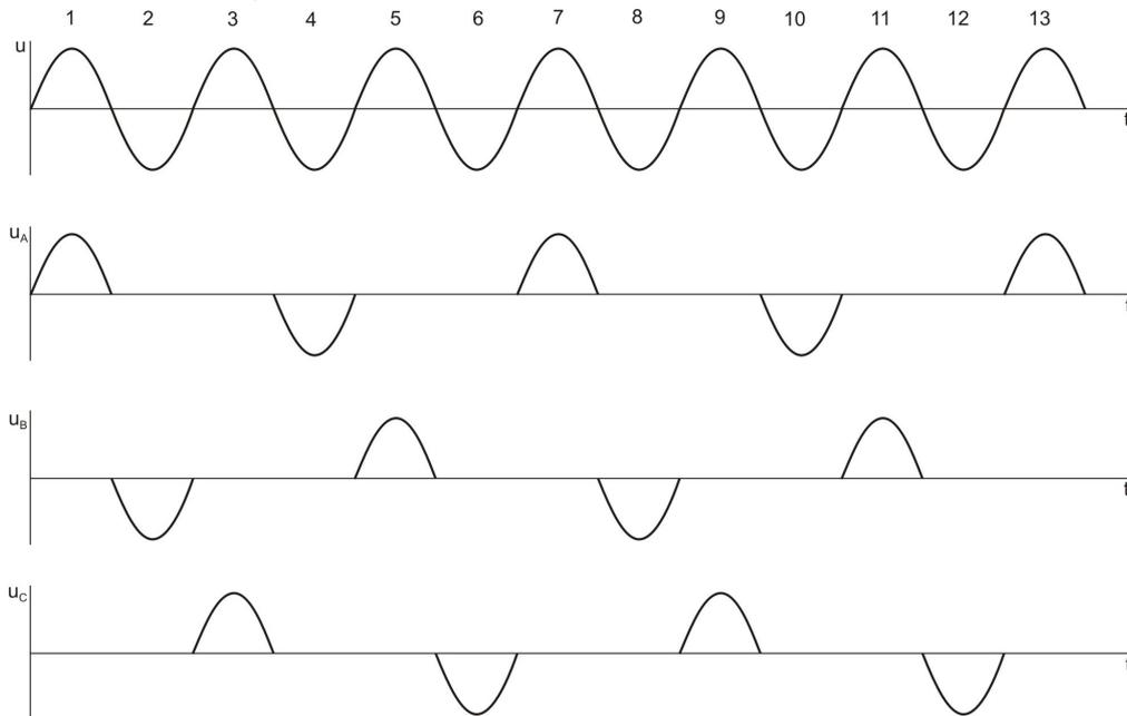
Fig. 1. The voltages of stator windings distribution
