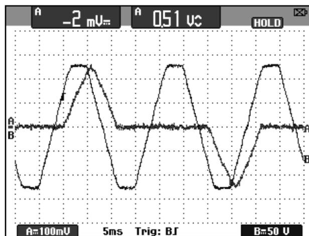
Fig. 3. Oscillogram of stator winding current and voltage:
